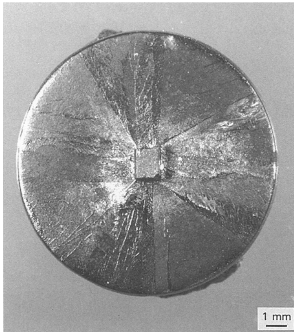
Figure 10 A photograph illustrating the morphology of a seeded melt-textured specimen. The specimen was melted under an optimized heating rate of 10^{\circ}\text{C h}^{-1} .
